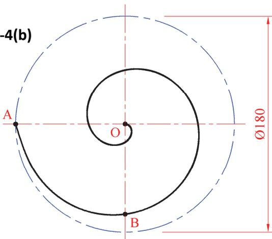
Fig C-4(b) on the left shows the projections of an inverted cone. An Archimedean Spiral moves clockwise from **O** to **A** in 1.5 revolutions, as shown in plan.
