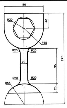
A design for a **TROPHY** is shown. Reproduce the given figure, showing clearly all constructions and points of contact.
