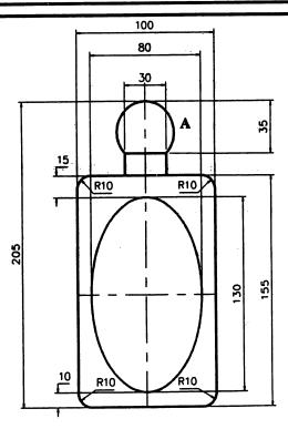
The figure shows the design for a **PERFUME BOTTLE**, with a label, in the shape of an **ELLIPSE**. Draw **FULL SIZE** the given design showing clearly how the centre for the arc A is obtained.
