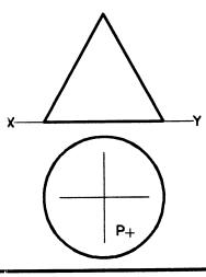
12. Shown are the orthographic views of a container. The container is <u>open at the top</u>. Draw the surface development of the container.
