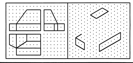
9. Shown is the elevation and plan of a solid. Complete the auxiliary plan of the solid on the given  $X_1 - Y_1$  which will show the true shape of the surface S.
