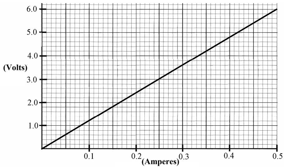
Use this graph to *calculate the resistance* of resistor **R** shown in the diagram.
