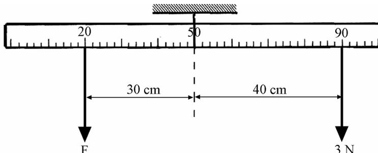
The diagram shows a metre stick suspended from its centre of gravity. A force of 3 N acts on the stick at the 90 cm mark and a force of  $F$  N acts on the stick at the 20 cm mark. The metre stick is balanced horizontally. Calculate *force F*. (6)
