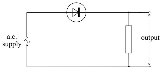
The diagram shows a p-n diode being used as a half-wave rectifier.
