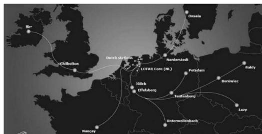
I-LOFAR links into the international LOFAR network, which comprises thousands of antennae that record measurements at the lowest frequencies that can be observed from the Earth. This network comprises 51 stations and is the largest virtual radio telescope dish in the world; it has a diameter of 2000 km. Each station connects to a central core in the Netherlands via high-speed fibre optic cable.
