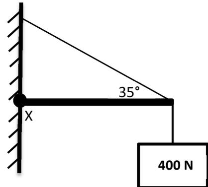
Calculate the clockwise moment acting on the rod (due to the weight of the sign and the weight of the rod) about X.
