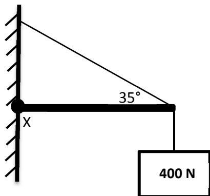
Calculate the clockwise moment acting on the rod (due to the weight of the sign and the weight of the rod) about X.
