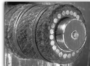
The first successful transatlantic cable connected Valentia Island, Kerry with Newfoundland, Canada in 1866. Many new electrical devices were used in the enterprise, including the Wheatstone bridge, which measured variations of resistance to locate breaks in the cable. The time taken to transmit messages across the Atlantic had been reduced from weeks to seconds.
