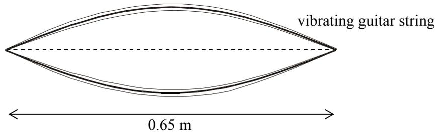
The diagram shows a guitar string stretched between supports 0.65 m apart. The string is vibrating at its first harmonic. The speed of sound in the string is  $500 \text{ m s}^{-1}$ . What is the frequency of vibration of the string? (9)
