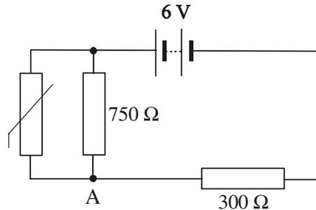
In the circuit diagram, the resistance of the thermistor at room temperature is  $500 \Omega$ .
