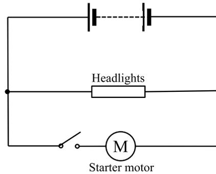
In the diagram, a car battery has an e.m.f. of 13.75 V and an internal resistance of 0.08  $\Omega$ . The effective resistance of the car headlights is 1.50  $\Omega$  and the effective resistance of the starter motor is 0.20  $\Omega$ . Calculate:
