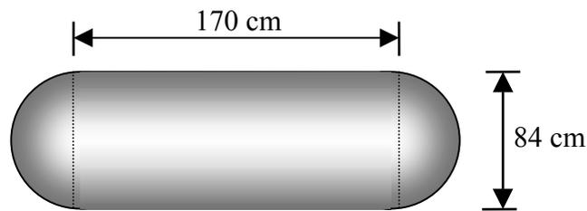
A capsule is made up of a cylindrical section and two hemispherical ends. The length of the cylindrical section is 170 cm and the diameter is 84 cm.
