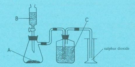
Dry sulphur dioxide is prepared in the laboratory by using the apparatus shown above.
