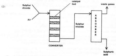
The diagram shows a simplified outline of an industrial plant for the manufacture of sulphuric acid by the Contact process.
