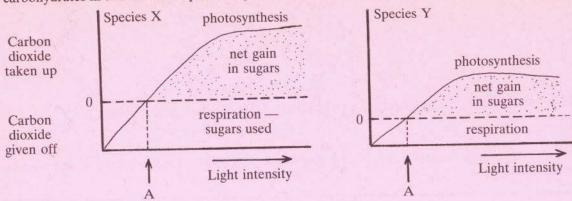
What term is used to describe the level of light intensity at the points marked A? Briefly explain the meaning of this term.
