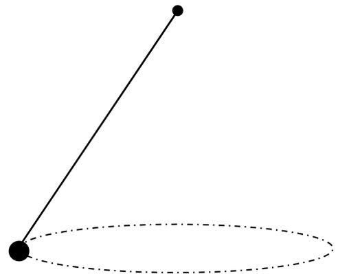
9. A right circular cone of radius 12 cm and height 25 cm is placed at the bottom of a tank of water. A sphere, of radius 4 cm is attached to the top of the cone with a light inelastic string. The relative density of the cone is 1.8 and the relative density of the sphere is 0.7.
