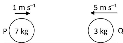
The coefficient of restitution for the collision is  $\frac{2}{3}$ .
