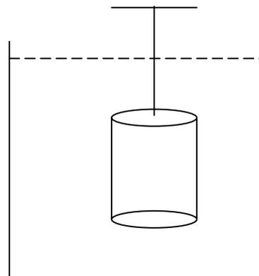
The cylinder is held at rest by a light inelastic string which is attached to a fixed support. The top of the cylinder is horizontal as shown in the diagram.
