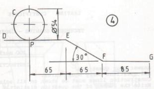
5. The elevation and plan of a solid which is to be cut by the oblique plane VTH are given in Fig. 5.
