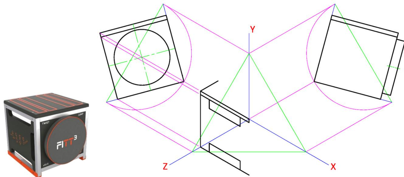
**A-3.** The graphic below shows a food product display marker used in a cafe. The incomplete drawing below shows the plan of the display marker and the oblique plane **VTH** which contains surface **S**.
