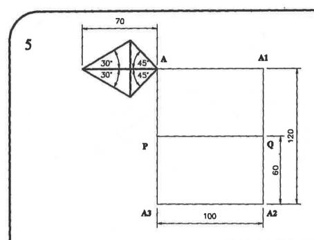
Draw the given figure and complete the rectangle 100 mm x 120mm as shown. Find the image of the given figure under the following transformations:-
