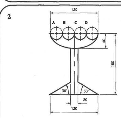
A design for an ORNAMENT based on a semi-ellipse is shown. The Major Axis is 130mm and the Minor Axis 80mm. Draw full size the given design showing clearly how the centres for the 4 circles A,B,C and D are obtained.
