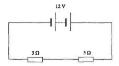
Calculate the value of the current which flows in the circuit.
