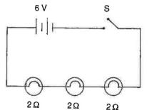
The diagram shows three lamps connected to a 6 volt battery in a circuit. Calculate:
