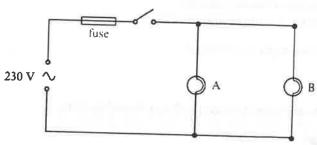
A is a 75 W lamp. The switch is closed. Calculate the current flowing through lamp A.
