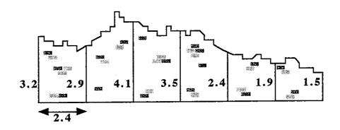
All distances are measured in metres. The heights are measured at intervals of 2.4 m along the base line.
