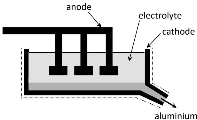
Alumina ( $\text{Al}_2\text{O}_3$ ) is exported from Ireland to be processed into pure aluminium by the electrolysis of the molten oxide in a cell similar to that shown in the diagram above.
