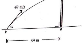
Find also the horizontal distance from k of a second vertical pole of the same height, so positioned that the particle again just passes over the top of it.
