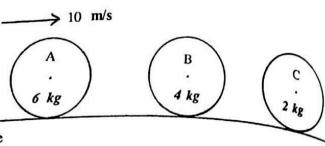
A is projected at 10 m/s so as to collide directly with B. As a result of this collision B moves forward to collide directly with C.
