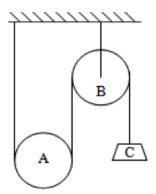
When the system is released from rest show that the acceleration of the particle is  $2m/s^2$  and that the acceleration of the pulley is half this. Find also the tension in the string.
