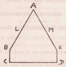
If the triangular portion ALM is removed (AL=AM= 2cms.), find the distance from CD of the centre of gravity of the remainder.
